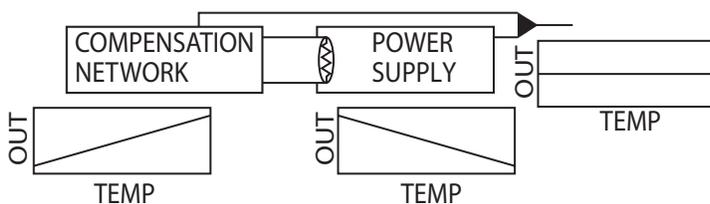
Assume the following component has the given R-T transfer characteristics. By incorporating the thermistor into the component biasing circuit, the effects of component temperature rise can be negated.
