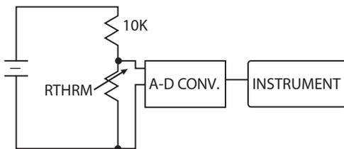
Figure 1. (Left) A thermistor/resistor voltage divider bridge can supply a strong signal to an A-D converter, which can then be interfaced to the desired instrument.
