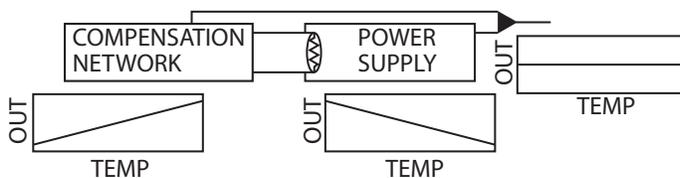
Assume the following component has the given R-T transfer characteristics. By incorporating the thermistor into the component biasing circuit, the effects of component temperature rise can be negated.
